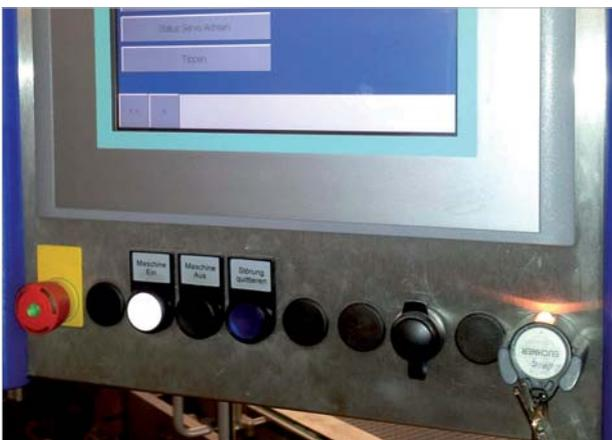
On the right side of the operating unit: the modular Electronic-Key adapter of EKS Light.
