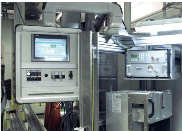
Illustration 2: The Electronic-Key is inserted in the Electronic-Key adapter of the EKS Light (right)
